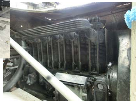
Ever see a 6 cylinder Air Cooled Diesel truck engine?
