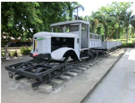
This track maintenance rail vehicle was adapted from a commercial diesel truck.
