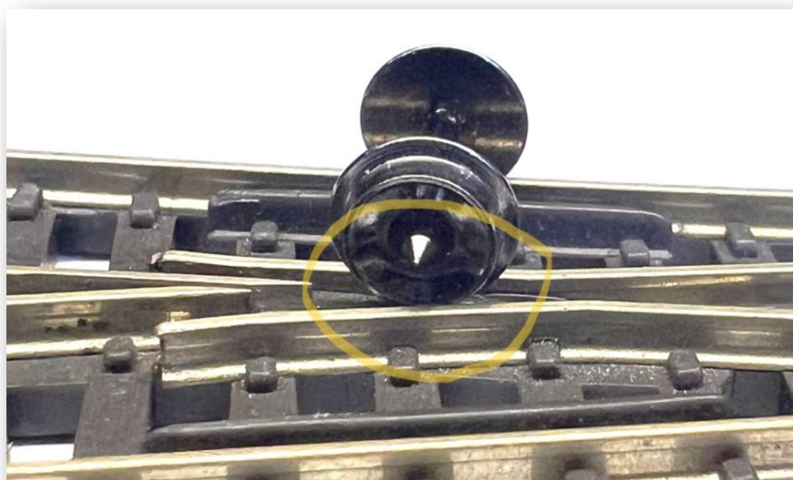
Figure 1: Metal Wheel drops into flangeway at frog.
