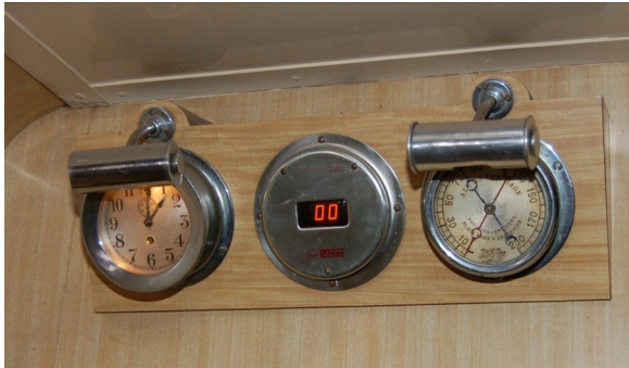
From Right to Left: Clock, Speedometer, Air Brake Gauge (Red Dial: Cylinder Pressure, Black Dial: Pipe Pressure)
