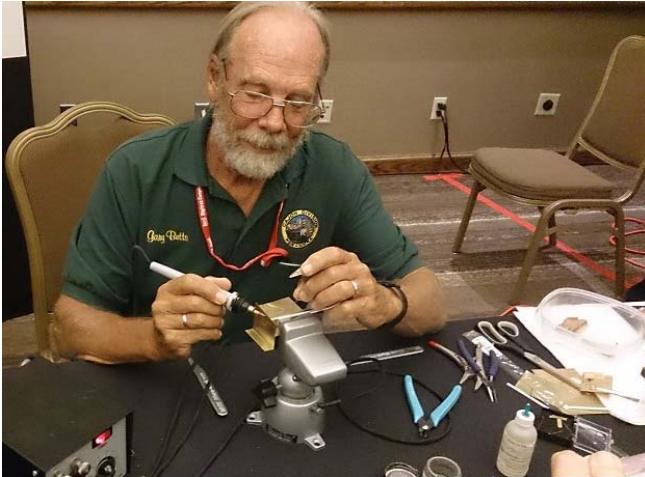
Gary Butts showing resistance soldering
