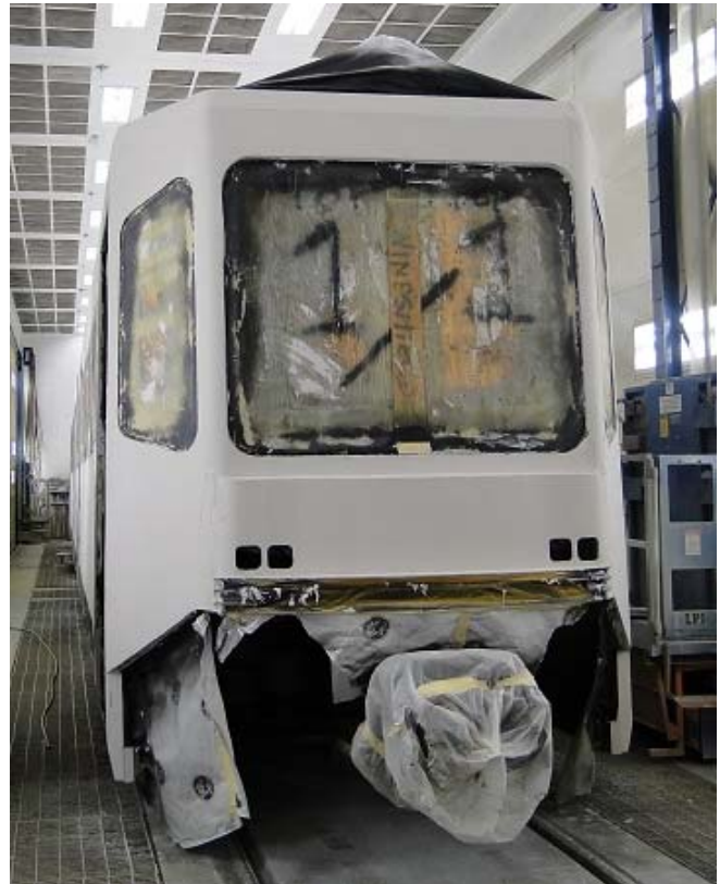
A MAX Type 1 LRV in the paint booth with the second of 7 coats applied
