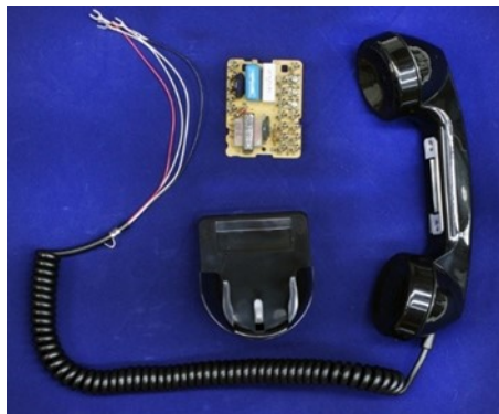
Figure 2 Basic Phone Component Kit
