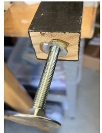
***Figure 3 – Elevator Bolts***
