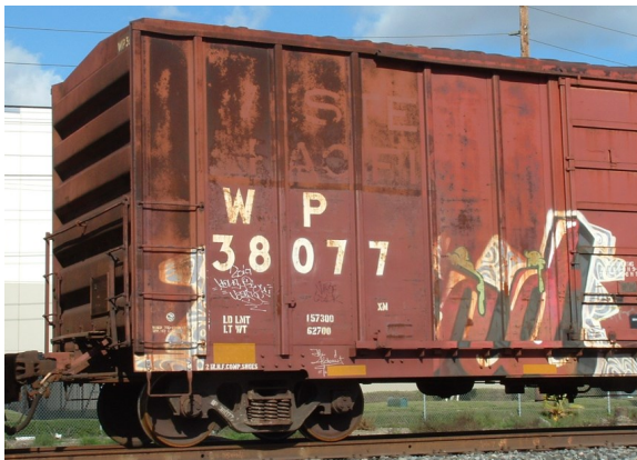
Near end of life and stored in Pomona, CA. WP 38077 note the level 3 paint and rust showing up.
