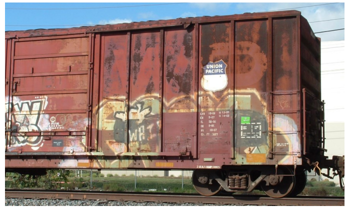
Another patch of new paint to cover tagging for the dimension details to be readable. The truck is faded gray and springs are showing slight orange-brown for rust color. Old large WP lettering is ghosting through above paint patch.
